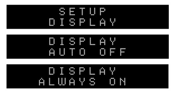
As for the balance, this feature is applied in real-time to give user the possibility to immediately see the results; a short message indicating the present setting appears on the display when the "DIM" key is used.
